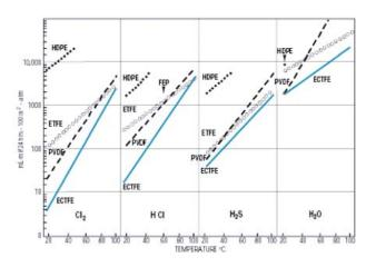
The electrostatic powder coated Halar® shows superior performance than conventional Fluoropolymers that can be shown with more information available in our Data Base on request.
